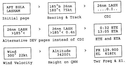
Note: Wind velocity is only shown if the compass option is installed.
