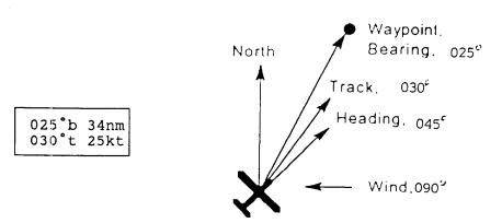
The locator on the main screen will be showing one 'turn left' arrow to indicate the 5° difference between the bearing and track. If the glider is turned 5° left, the bearing and track will now be the same and only the central bar denoting 'on track' will be shown on the locator. The glider is then tracking directly to the TP with an allowance made for any cross wind.
